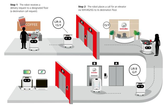
**Step 4**: Upon task completion, the robot will return to the docking.
